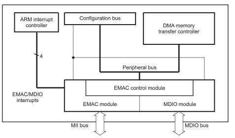
Figure 1. EMAC and MDIO Block Diagram
